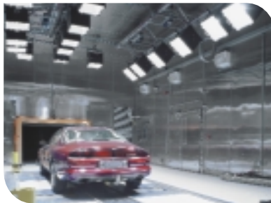
SolarConstant in a solar evening configuration
