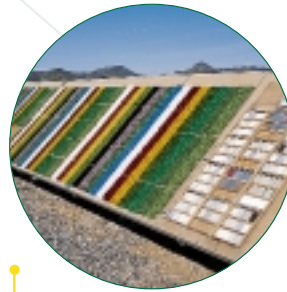
45° backed rack— central Arizona
